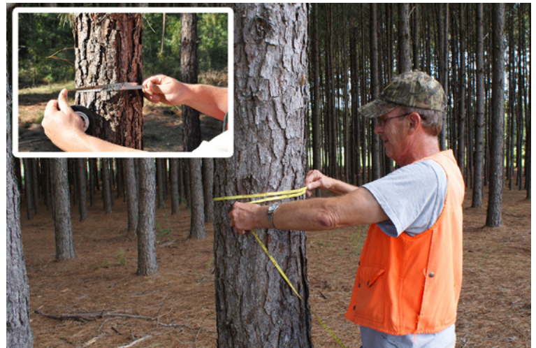
Figure 2. Measuring tree diameter (DBH) with a diameter-measuring tape.
