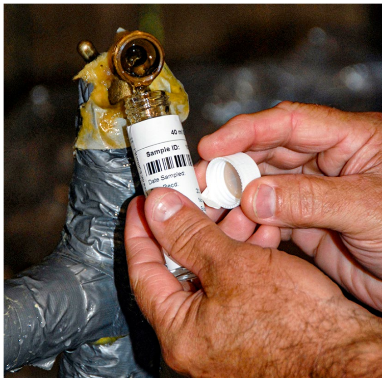
Figure 3. Use only the container provided by the testing laboratory for taking well-water samples.
