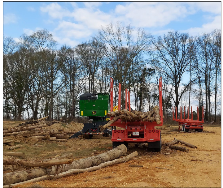
Figure 6. Trainees can pair operation on the simulator with running actual equipment at the Hinds County Community College Logging Equipment Operator Program field site owned by the Mississippi Forestry Commission. Shown in the upper picture is a John Deere 848L-II grapple skidder, while the lower picture contains a John Deere 337E loader (with a pull-through delimeter) and two Fryfogle Manufacturing Inc. four-bolster logging trailers.
