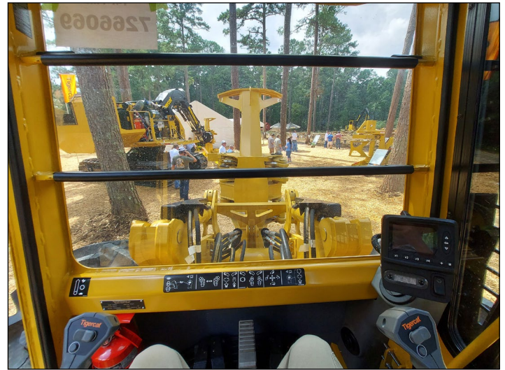
Figure 1. This is a modern, wheeled—or drive-to-tree—feller buncher. Notice the control levers (very similar to joysticks) and buttons to operate various processes of the feller buncher. There is also a GPS unit on the right side.
