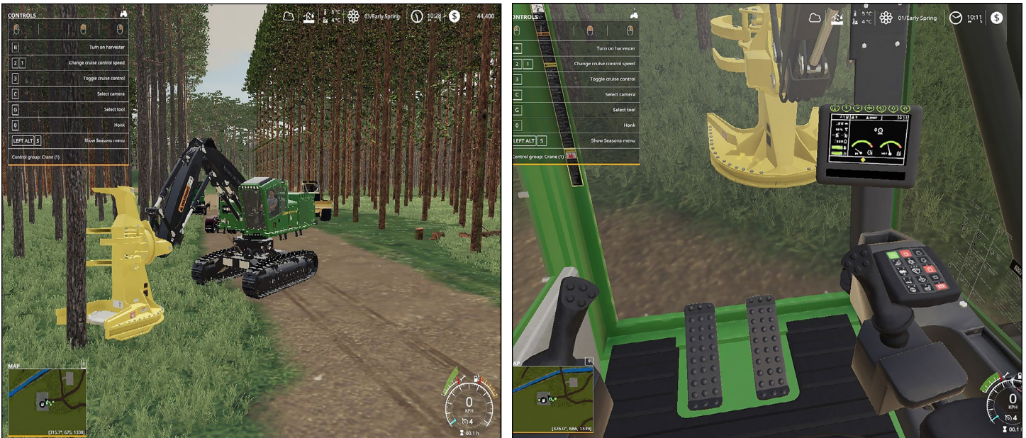
Figure 4. A simulated tracked feller buncher within Farming Simulator 19 (FS19). Farming Simulator 19 and 22 provide fairly sophisticated representations of actual logging equipment and different forested conditions within a video game platform. Users can select from many different types of equipment and actual manufacturers, including common equipment such as drive-to-tree (wheeled) feller bunchers, wheeled skidders, loaders, tracked processors, and pull-through delimiters.
